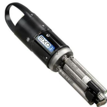
Possible extension (example): EXO3S multiparameter sonde
