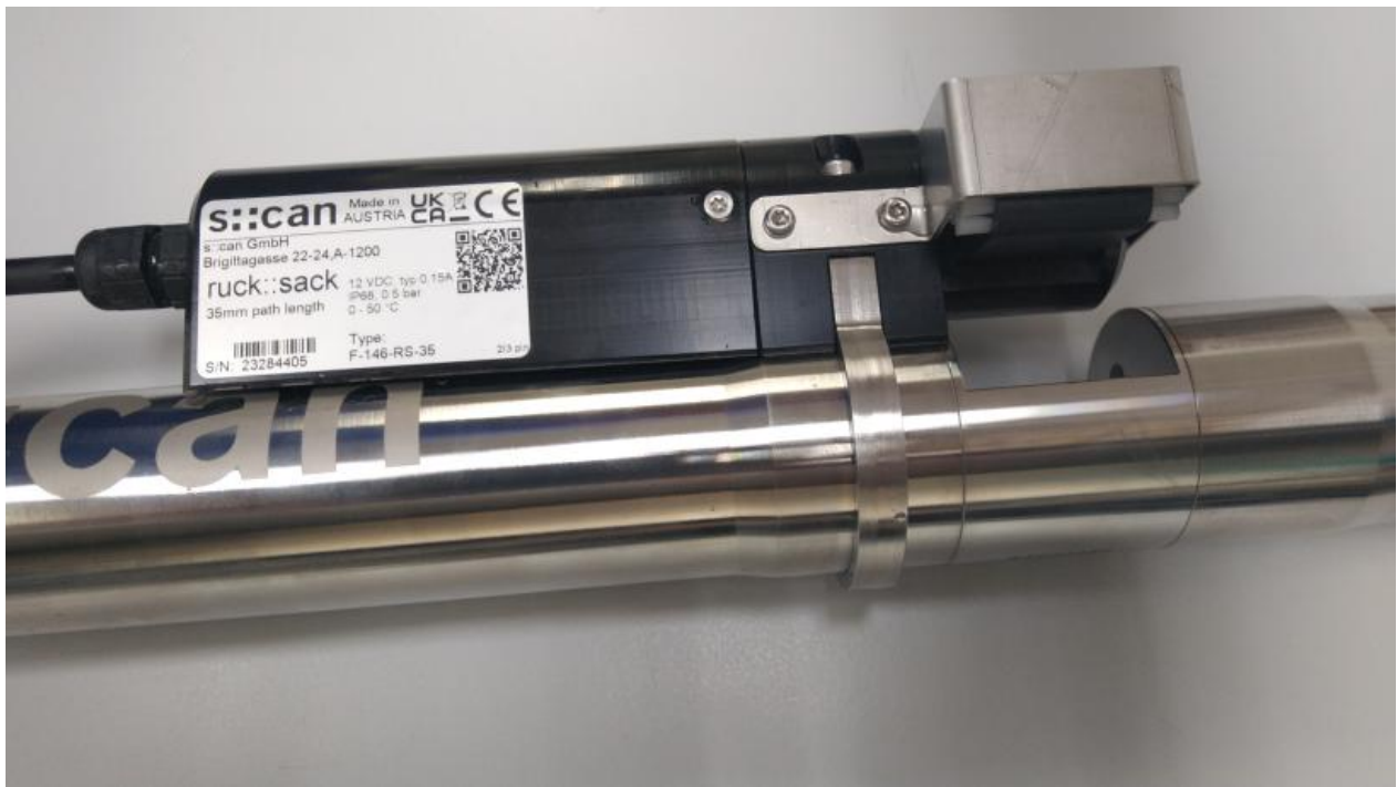
Figure 23. The ruck::sack mounted on a spectroyser (both from s::can).
