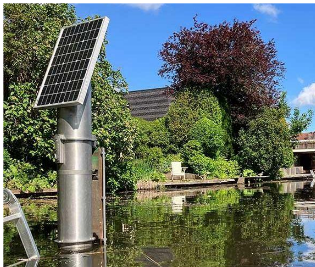
OMC-048 in a vandalism-resistant pole for water quality monitoring.
