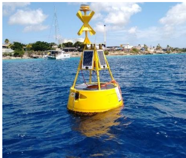
OMC-048 in a data buoy for water quality monitoring.
