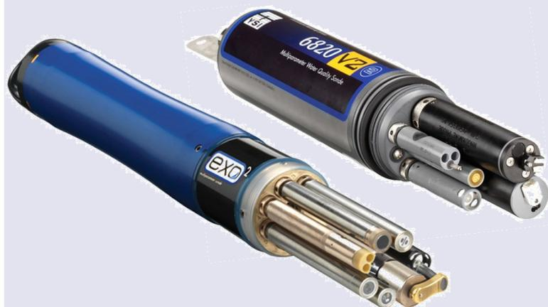
*YSI/Xylem Multiparameter probes. EXO series and 6-series.*
