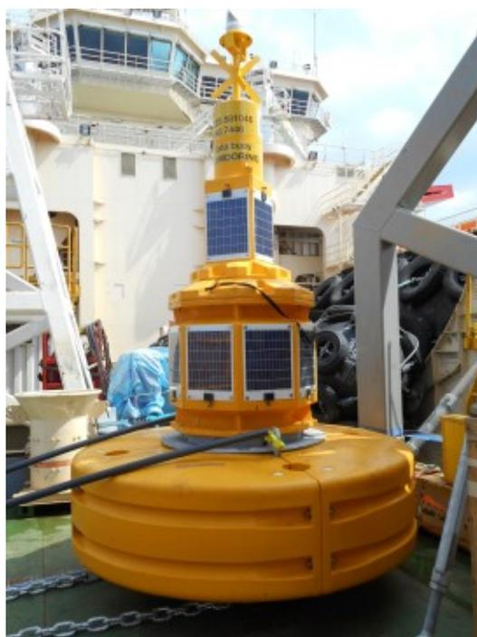
OMC-7018 Data buoy for wave, water current, water quality and meteorological parameters.
