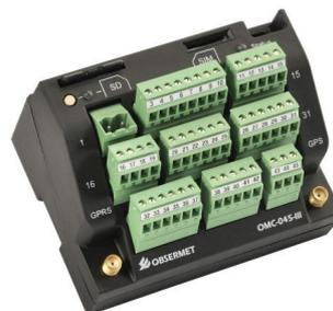
*OMC-045-III data logger with integrated GPRS and GPS*
