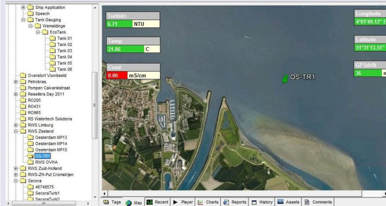
Fig. 5: Example screenshot. The left pane shows how sites are hierarchically organized. The right pane shows the selected location in a number of tabs. The 'map'-tab shows the location of a data buoy (OS-TR1).
