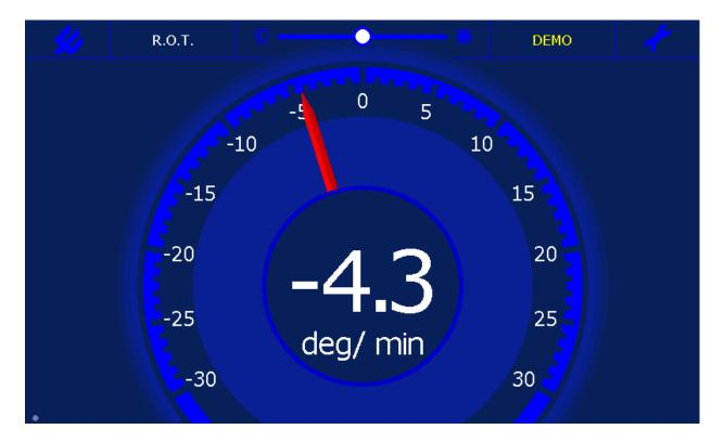
This screen displays the Rate Of Turn (derived from the gyro) as a dial gauge and numeric in the middle.
