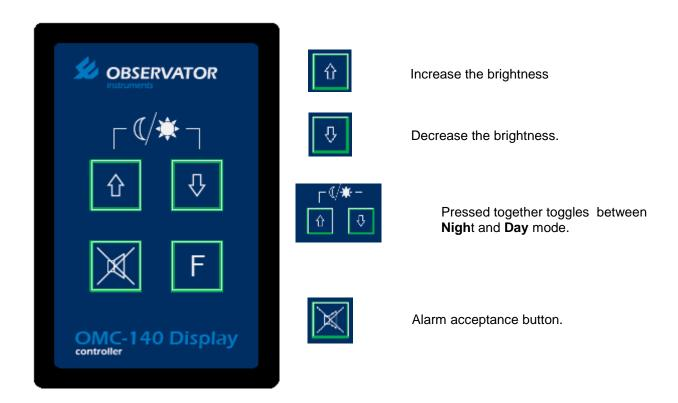
Default the remote is in Brightness control mode. If no button press has been detected for 10 seconds it will return to this mode.
