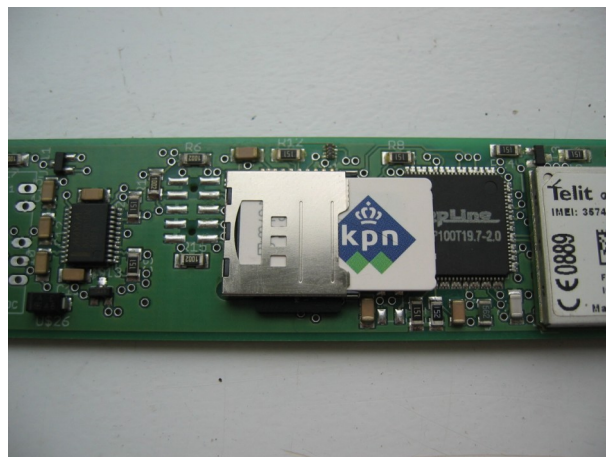
SIM card installed on PCB, 2 GB Micro SD memory card is positioned under SIM card holder.
