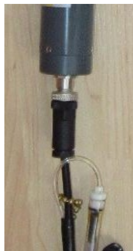
INW connector (IP67) installed on tube housing.
