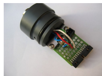
OMC-040 main board (above) and connection board with bottom part (left)
