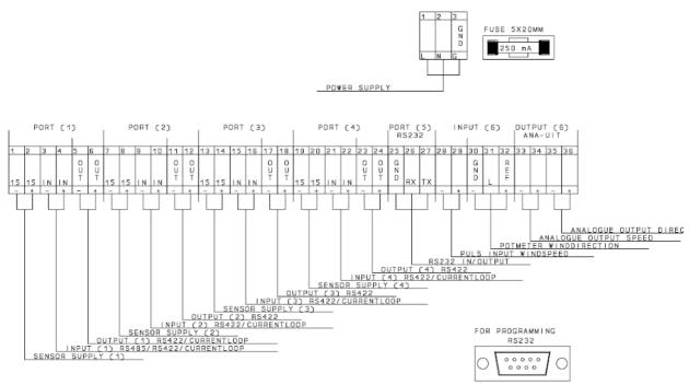
If the Observator Instruments wind sensors are used, the terminals 1. 2. 3, and 4 are used for sensor 1 and the numbers 7, 8, 9 and 10 for sensor number 2.
