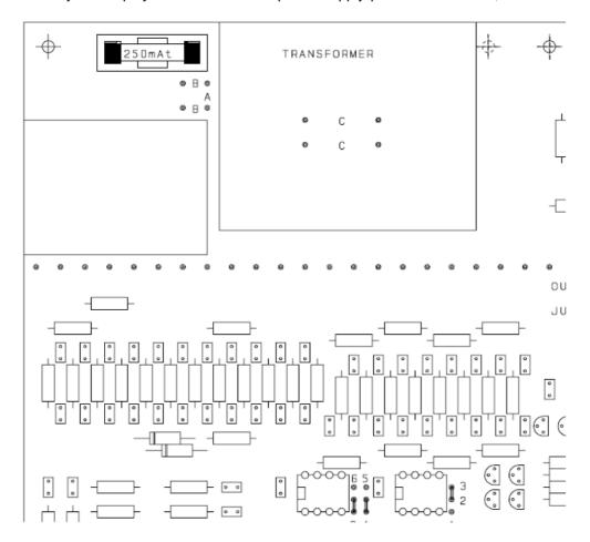
On the power supply board, the PCB with the terminal connection on the rear side, there is installed a transformer. The transformer offers the possibility of 115 or 230 Vac. The supply depends on the jumper settings between the filter transformer and the supply transformer. (See PCB layout) If the wired marked "B" are installed the unit is set for 115 Vac, If the wire "A" is installed the unit is set for 230 Vac.
