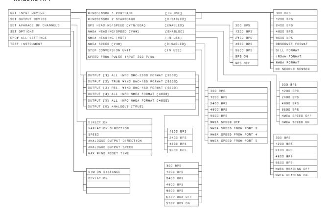
Select the proper transmission speed, the speed is as a standard set to 9600 bps. This setting might be set differently, if no response from the instrument when pressing the ENTER button on the keyboard try a different transmission speed.
