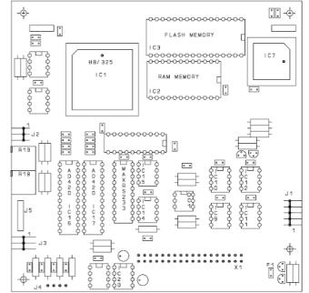
the correct sockets. For the analogue output the following IC,s have to be installed, IC16, IC17, IC18 and IC20. To select the correct output signal see above for the correct jumper settings.
