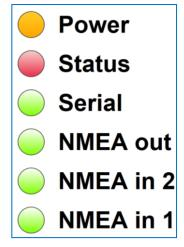
If you experience difficulties connecting with the device; Check if the LED's are blinking, Check the wiring of the Tx/Rx or A/B wires; Check the data settings of your COM port.
