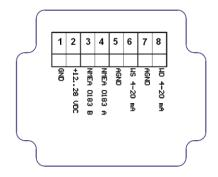
Recommended cable: shielded 2x2x0,75mm2 twisted pair
