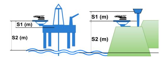
Always use the height of the location of the barometric sensor itself, even if a pressure head (OMC-509) is used. The location of the pressure head is irrelevant for the sensor height! The sensor is preferable build in the same housing as the OMC-183-ML.
