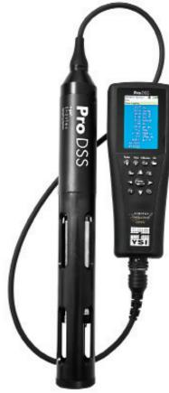
Parameters: Dissolved Oxygen (Optical) **Turbidity** рH ORP/Redox Conductivity **Specific Conductance** Salinity Total Dissolved Solids (TDS) Resistivity **Seawater Density** Total Suspended Solids (TSS) Depth Ammonium Ammonia Chloride Nitrate
