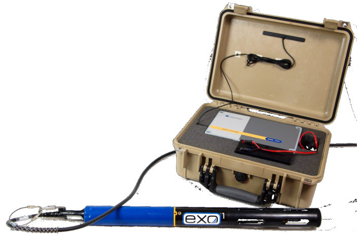
OMC-045-III datalogger and YSI-EXO Multi-parameter sonde.
