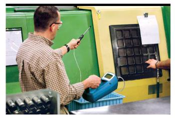
P-Trak Ultrafine Particle Counter and accessories includes: Telescoping Sample Probe, Shoulder Strap, Inlet Screen, Spare Wicks (2), Alkaline Batteries, Alcohol Fill Capsule with Storage Cap, Reagent Grade Isopropyl Alcohol, Zero Filters (2), Carrying Case, TrakPro<sup>m</sup> Software, Computer Cable, Operation and Service Manual, Calibration Certificate, and Two-year Warranty.
