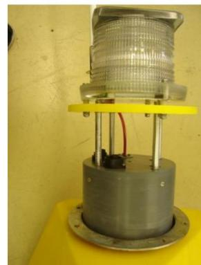
The contents of the water-tight container. The OMC-045-III logger is clearly visible. The water-tight container slides from the top into the buoy.
