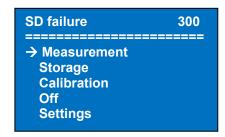
If the SD-card is removed during the writing of data an error "SD failure 300" will occur. The number at the right will count down. It is possible to reinsert the SD-card while the counter is still active. The data will still be saved. Not reinserting the SD-card will result in data loss.
