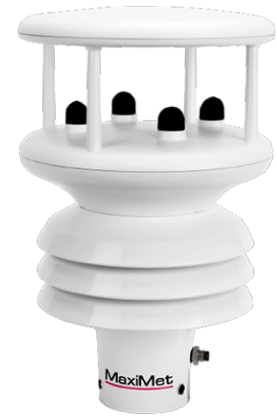
MaxiMet GMX550 measures 6 parameters including precipitation
