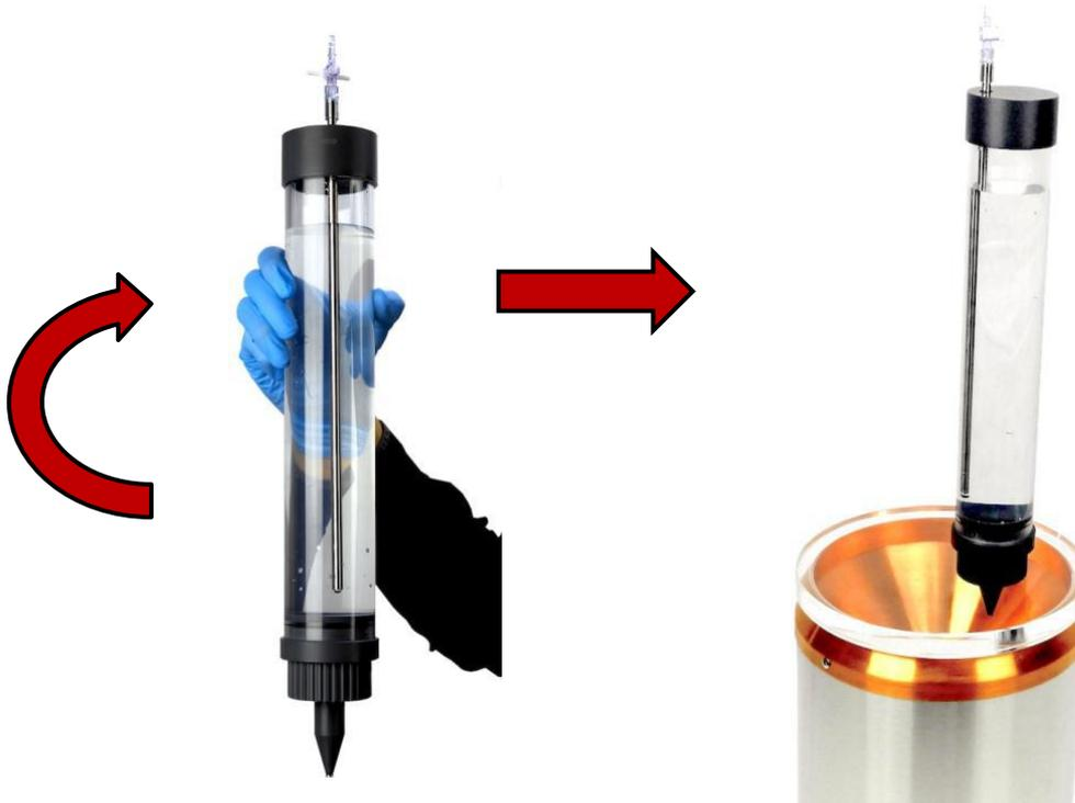
5. Open the siphon valve. The water will flow out of the RIM-FVU to the tipping bucket rain gauge at a predetermined rate. The number of tips can either be audibly counted or digitally counted (these can be bought as an option), or the counts can be retrieved from a data logger and checked against calibration specifications.
