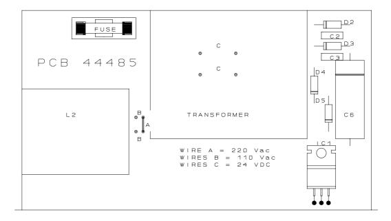
As an option the OMC-934 can be delivered for 12 Vdc, If the unit has to be modified to work with 12 Vdc the transformer has to be removed. With the transformer removed it becomes possible to install a DC/DC converter on the location of the transformer. The DC/DC converter converts the 12 Volt supply voltage up to 24 Vdc.
