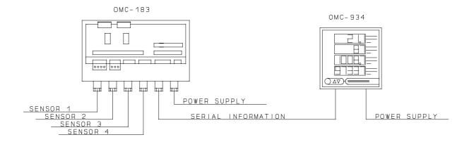
If more than 4 sensor are connected a second OMC-934 can be connected via the daisy chain output of the first display.
