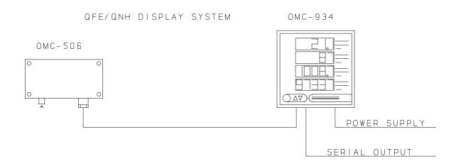
Parameters needed to calculate the QFE and the QNH can be set via the RS232 port on the rear of the instrument or via the buttons on the front panel. When the buttons "arrow-up" and "menu" are pressed simultaneously the instrument switches to the setup parameter mode. In the upper display the number of the parameter is shown, the second display shows the parameter digits for the decimal point the third display shows the parameter digits behind the decimal point.
