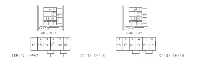
Recommended cable: 1 twisted pair with common screen, core size 0.75 mm2.
