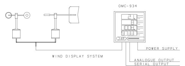
The range of the potentiometer and the pulse must be set in the factory or by the customer using the RS232 port at the rear of the instrument. When "Analogue
