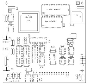
For the analogue output the following IC,s have to be installed, IC16, IC17, IC18 and IC20. To select the correct output signal see above for the correct jumper settings.
