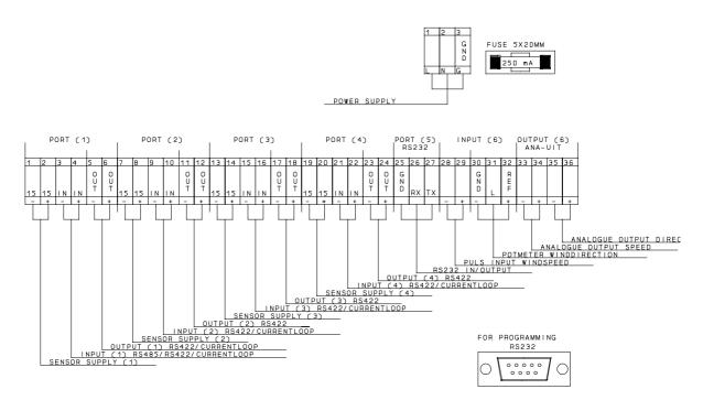
If the Obsermet windsensor is used, only the terminals 1. 2. 3, and 4 are used. Daisy chaining to the next instrument is done on the terminals 5 and 6.
