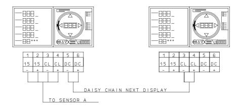
Recommended cable: 1 twisted pair with common screen, core size 0.75 mm2.
