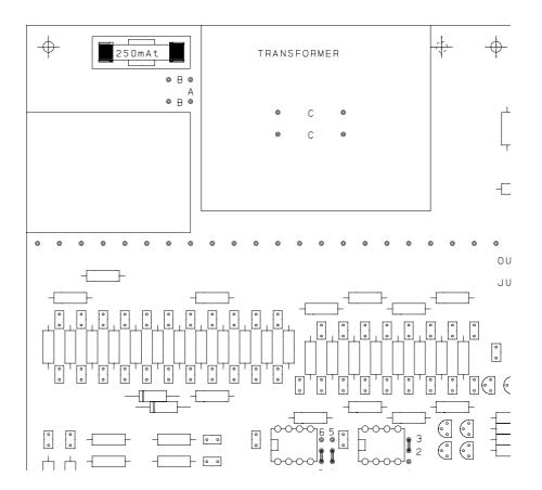
As an option the OMC-137 can be delivered for 12 Vdc, If the unit has to be modified to work with 12 Vdc the transformer has to be removed. With the transformer removed it becomes possible to install a DC/DC converter on the location of the transformer. The DC/DC converter converts the 12 Volt supply voltage up to 24 Vdc.
