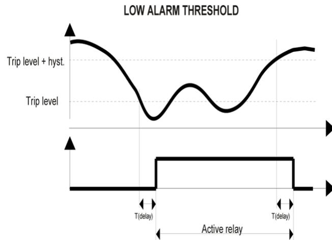
So, the entry of an alarm state is NOT affected by a hysteresis. Hysteresis is only used for switching back to the normal mode. The amount of hysteresis has an effect on the “sensibility” of the alarming. It is strongly advised to use a certain amount of hysteresis to prevent from multiple alarming warnings. The amount of hysteresis is determined by experience and information from the sensor.
