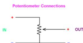
The output voltage is adjustable from 0% to 100% of  $V_{in}$ , in this case. The OMC-043 data logger has 3 terminals (on connector X1) for connecting a potentiometer to the logger:
