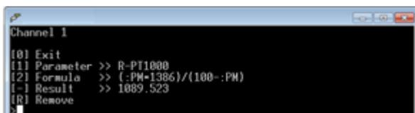
5) Create a calculated channel (TPT) to calculate the temperature of the PT1000 by entering the following equation:  $(:RPT - 1000) / 3.84$
