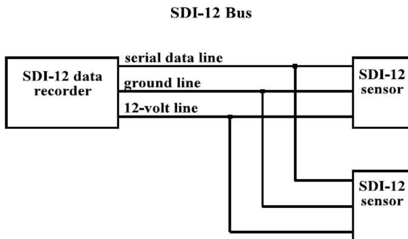
The wiring length between a sensor and the data-recorder must not exceed 60 meters. The maximum number of sensor connected to a SDI-12 bus is limited to 10. The data logger is protected against transients on the SDI-12 bus.
