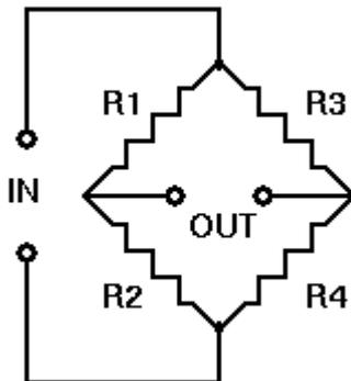
Given, all R's are the same the output voltage will be 0 Volts. In practice, one of the resistors is replaced by a variable resistor (often a strain gauge). By varying the resistance of this resistor, the bridge will be "unbalanced" and there will be an output Voltage, other than 0 Volts. To enable the circuit, the bridge has to be powered by a very stable reference Voltage, often called "Excitation Voltage". The OMC-042 has an Excitation output for this purpose.
