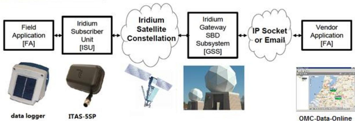
SBD messages are transmitted to an Iridium server (GSS: Gateway Short Burst Data Subsystem) and you can ask your Iridium provider to pass SBD messages to an e-mail address of your choosing or via directIP to an IP-address/domain and TCP-port of your choosing. When using your own software you have to either pick-up and import the e-mails or implement a TCP-server to receive SBD messages.
