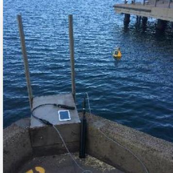
4. Allowances must be made for the effect of flowing water to ensure the stagnant depth rating is not exceeded. If the probe is to be installed downwards then it is recommended to install it a few degrees away from the vertical to allow bubbles to escape away from the optic face.
