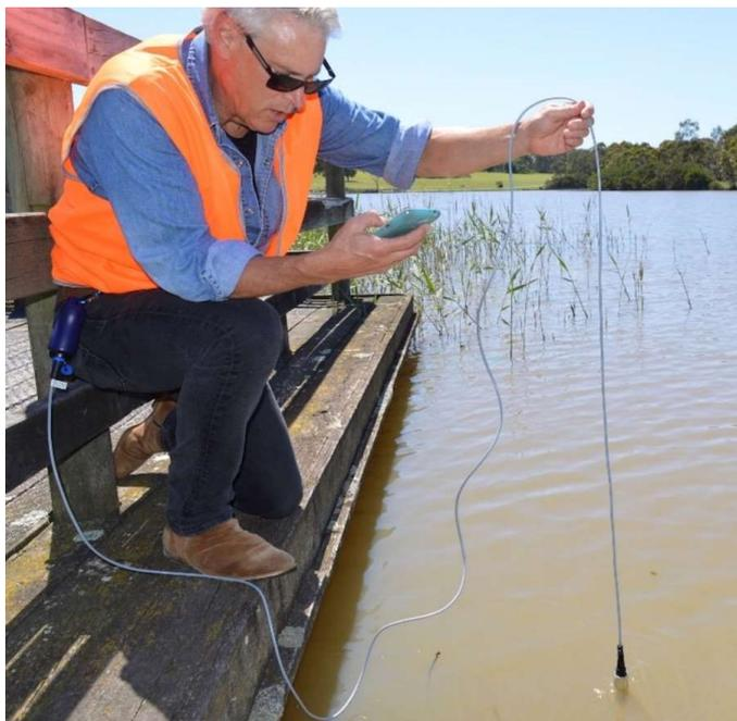
3. In a simple application the sensor is simply immersed into the water to the desired depth, but within the depth rating of the sensor. Please note the depth rating is based on stagnant water.
