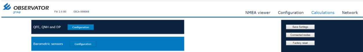
The Smart Node (OIC-05) can calculate the barometric pressure at sea level (QNH) and runway level (QFE).
