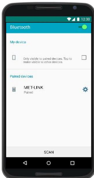
2. Go to the Bluetooth settings, scan to find the new device. Select the new sensor to pair and press pair.
