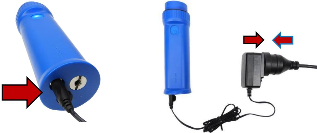
2. At any time, you can monitor the charging status of the module by pressing on the MET-LINK interface button. The LED indicator is flashing blue, green and red to indicate that the battery is charging.
