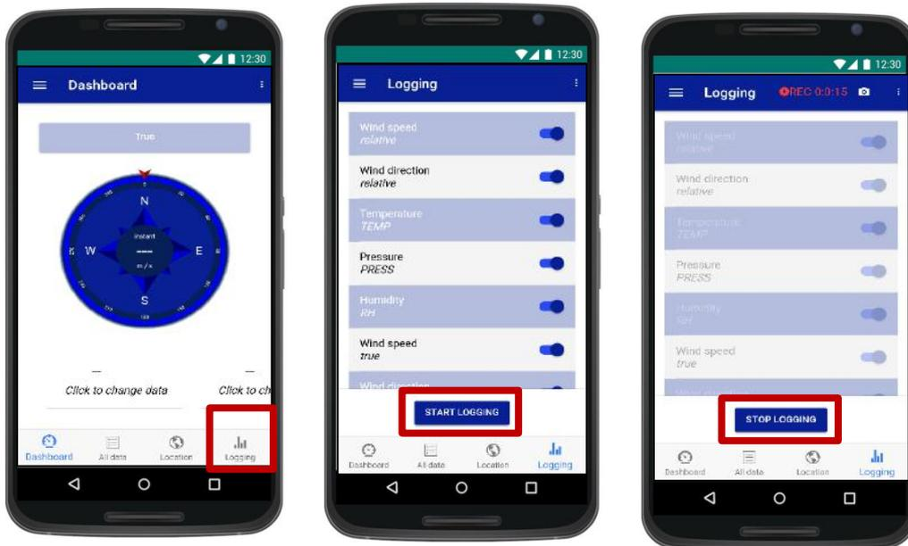
1. When connecting to the sensor for the first time, wait for few seconds in order to load the data and select "Logging" menu.
