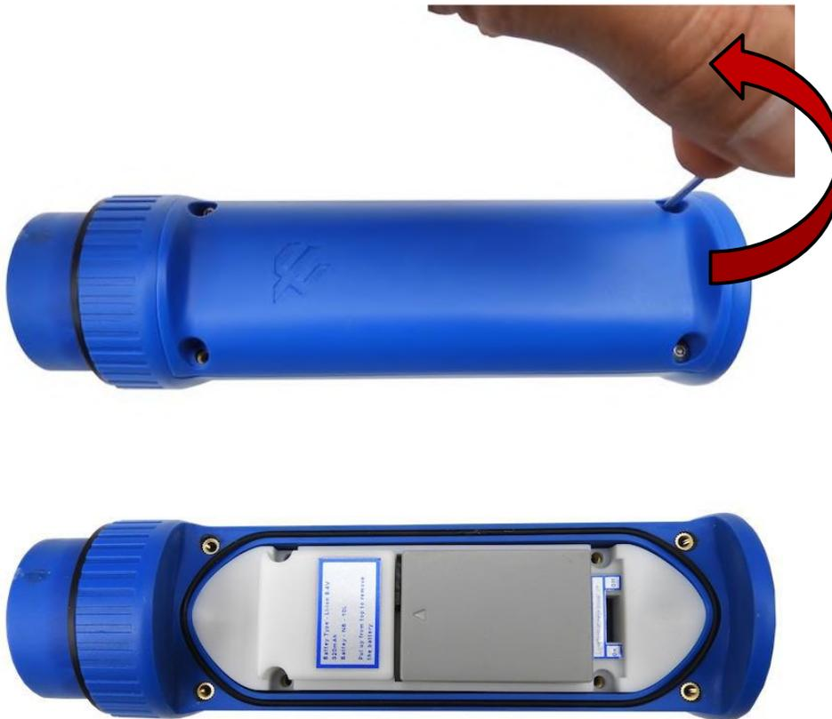
2. Disconnect the Lithium-Ion battery pack by pulling the battery up.
