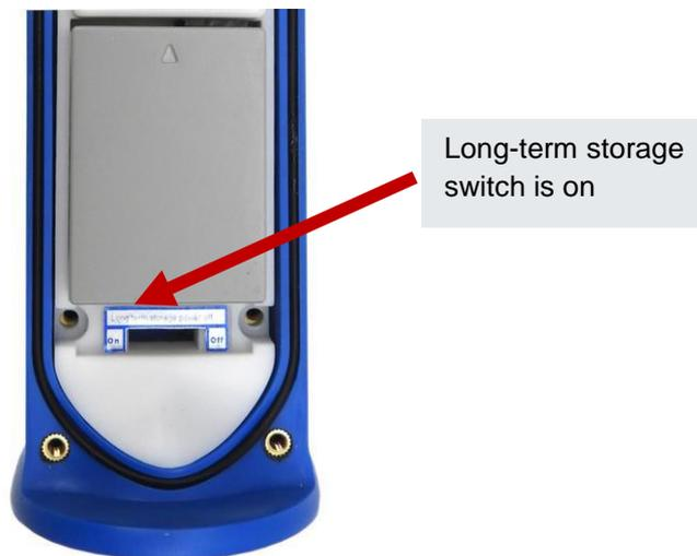
Connect the Li-Ion battery to the MET-LINK interface module (normally installed when provided). If not, please follow the instructions described in the **chapter 10: “Maintenance & calibration” section 10.1: “Battery replacement”**.
