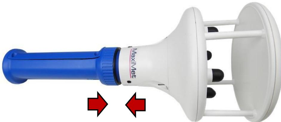
3. Press on the MET-LINK interface module button and notice the blue Light-Emitting Diode (LED) indicator is flashing. If you cannot see the blue flashing indicator light, it means the MET-LINK interface module is not powered.
