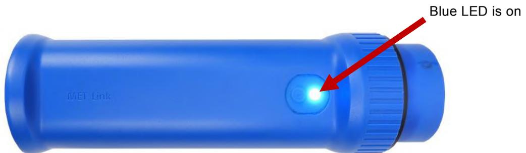
Note: In the event where the indicator is not lighting up, ensure that the MET-LINK interface module has enough battery (refer to the [“Charging the battery”](#) section 7.2 of this manual) and ensure that the long term storage switch inside the Bluetooth module is on.
