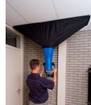
The **AT-242** is required for measuring supply and exhaust vents in residential housing. This light hood simply slides over the top of the Diff and doesn't require any additional tightening.
