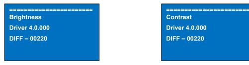
The screen gives information about the serial number and the driver number of the DIFF. The brightness or contrast is adjustable by turning the selection button. The setting can be confirmed by pressing the selection button.
