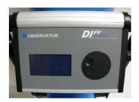
The DIFF can be switched on by pushing in the <u>middle</u> of the scroll button. The recess in the scroll button is intended for scrolling through the menu.
