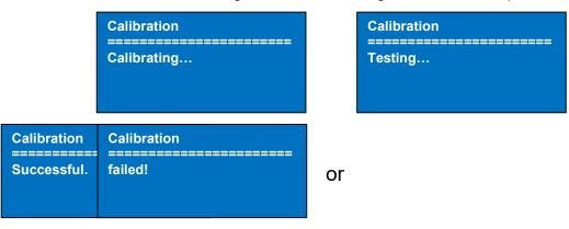
The last screen indicates that the calibration failed. The failure can be caused by air flows in the room. Make sure that the DIFF is calibrated on a flat surface. You can put a flat object on top of the DIFF to avoid airflow through the DIFF.
