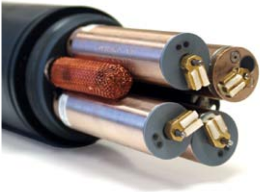
YSI 6600 sonde with installed anti-fouling kit
