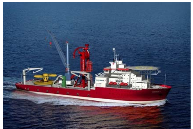
Deepwater pipelay vessel
