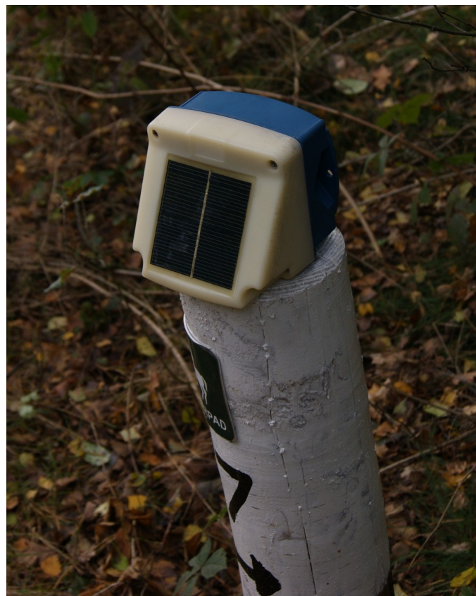
OMC-042-01 with integrated solar panel installed on top of a borehole
